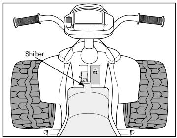
IMPORTANT! To avoid damaging the motors and gears, make sure to stop the vehicle before switching from drive to reverse.
